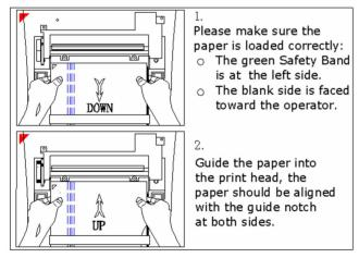
**Note:** Be careful when inserting paper. Avoid damaging the thermosensitive print head. Unless inserting paper or shooting troubles, do not leave the recorder door open.
