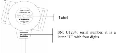
Figure 3.9 Label of ultrasound transducer
