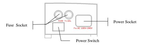
Power Switch (O/1): A.C. mains On/Off switch. O=Off, 1=On Fuse Specification: Size: Φ5mm\*20mm Model: T1.6AL 250V
