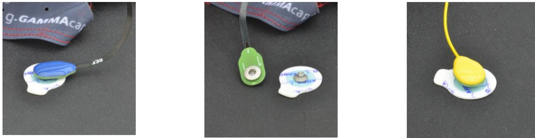
Left: reference electrode; Middle: Ag/AgCl snap-on electrode; Right: ground electrode
