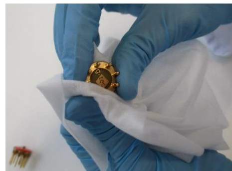
Figure 7: cleaning of the pins
