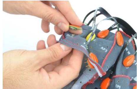
Figure 5: assembly and disassembly of the wires from the dry electrodes
