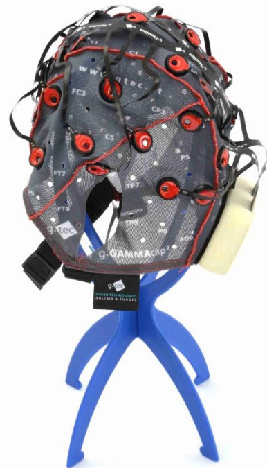
Figure 4: one example of a way to dry the wet electrode system
