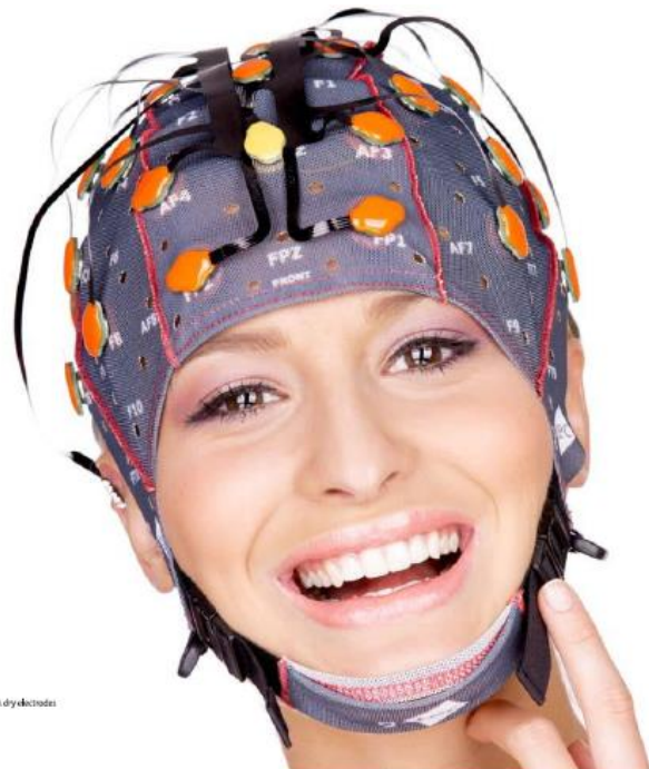
g.Nautilus PRO with 32 active dry electrodes
