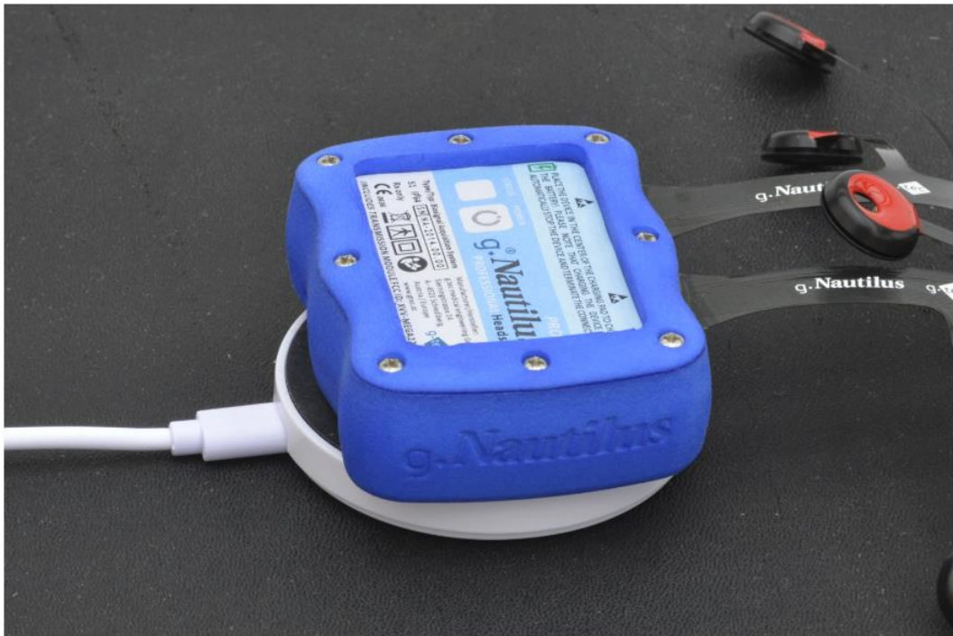
Charging of g.Nautilus Headset via a Qi-compatible charging pad.
