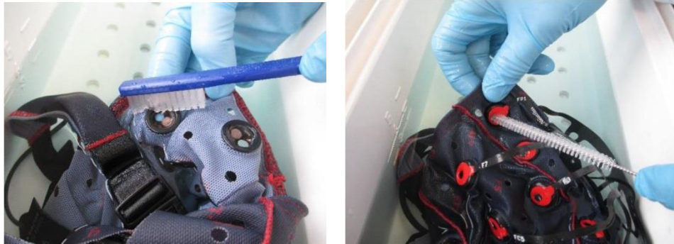
Figure 3: cleaning of the electrodes with the toothbrush
